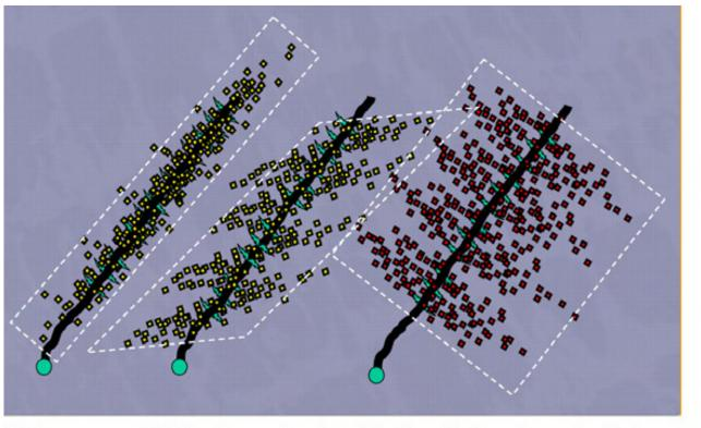
16. Importance of SRV and network azimuth for lateral orientation and well placement
