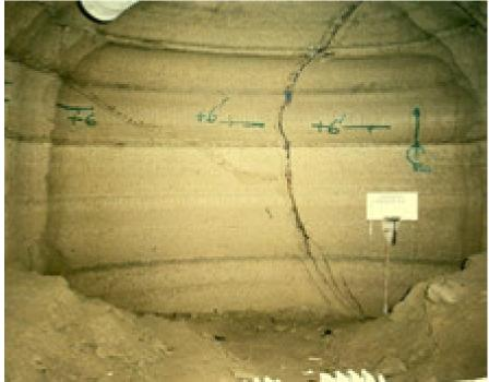
Warpinski, Sandia Labs. Nevada Test Site, Hydraulic Fracture Mineback
