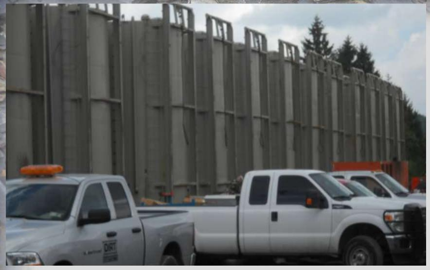
Vertical tanks provide more storage on size with less footprint, translating into smaller wells pads Marcellus Center for Outreach and Research
