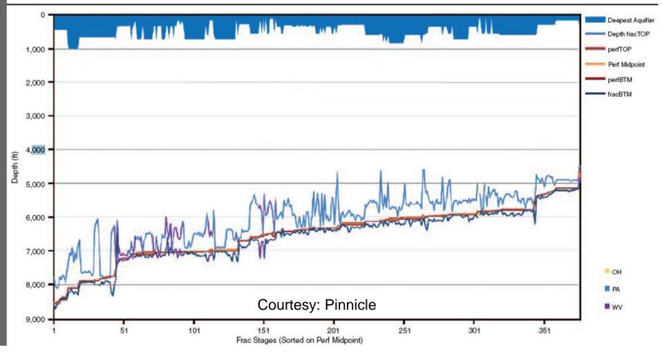
"Frac Barriers" of Onondaga Ls. below & Tully Ls. above. Marcellus Sh. thousands of feet below fresh water aquifers. Induced fractures cannot extend upwards because of overburden stress and horsepower limitations.
