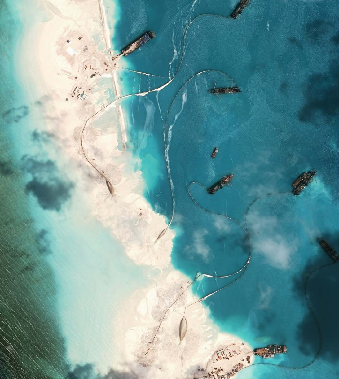
A satellite image captures Chinese efforts to create new islands through dredging up sand on Mischief Reef in the disputed Spratly Islands, which are claimed by China, Philippines, Taiwan, and Vietnam. China's actions in the South China Sea are an example of its assertiveness in its neighborhood. Image credit: CSIS Asia Maritime Transparency Initiative/DigitalGlobe.
