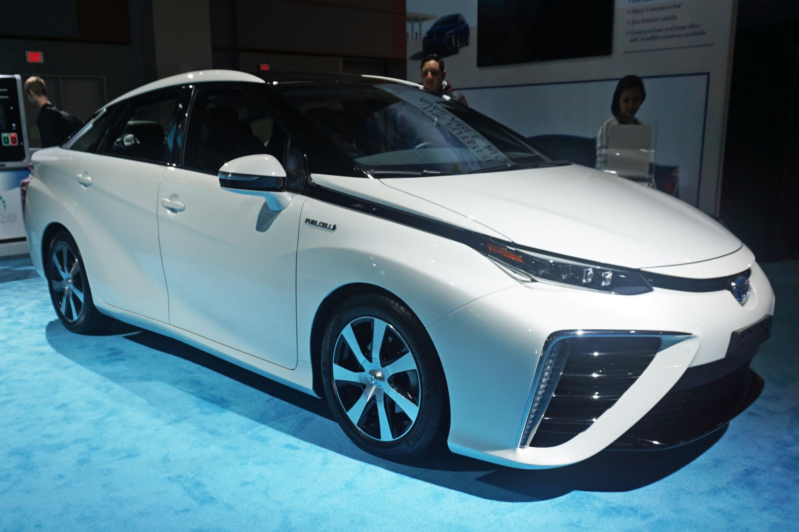
The 2017 Toyota Mirai, which uses hydrogen fuel cell technology, on display at the Washington Auto Show in Washington, DC. Initially launched in 2015, the 2018 Mirai is expected to have a 312 mile range and a combined fuel economy of 67MPGe (miles per gallon equivalent). Photo credit: Mariordo/Wikimedia.
