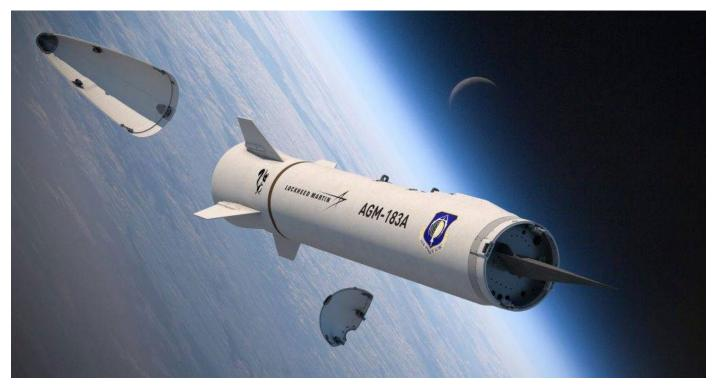
A boost-glide hypersonic weapon relies on a rocket to launch it into a low-Earth orbit, where the hypersonic projectile then detaches and glides on top of the atmosphere to its target. This design of the Air-Launched Rapid Response Weapon (ARRW) shows the rocket and projectile in low-Earth orbit prior to detachment. *Source: Lockheed Martin Corporation*
