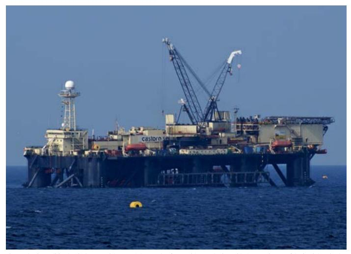
The semi-submersible pipe-laying vessel Castoro Sei operating for Nord Stream in the Baltic Sea south-east of Gotland, Sweden in late March 2011. *Photo credit:* Wikipedia/Philfaebuckie
