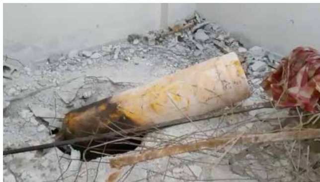
Remains of a chlorine gas cylinder at the balcony impact location in a video filmed on April 9, 2018 (Source – “Important: video from 9 April, 7:02pm showing presence of chemical gas canister in Douma. Same location as video of casualties. Also same location that Russia visited reporting ‘no sign of chemical weapons,’” Twitter, posted by The White Helmets, April 10, 2018, https://twitter.com/SyriaCivilDef/status/983768284133806080 )
