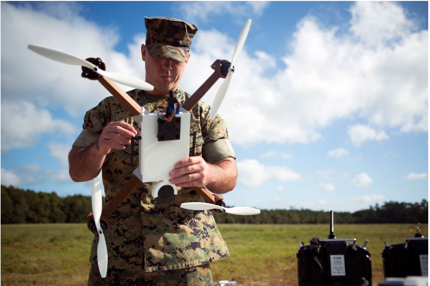
Marine Corps Lance Cpl. Nicholas D. Hettinga looks at a 3-D printed unmanned aircraft system at Camp Lejeune, N.C., Sept. 27, 2017. The drone was created through 3-D printing to be low cost, easily repaired and have simple maintenance. Photo Credit: Marine Corps photo by Cpl. John A. Hamilton Jr.
