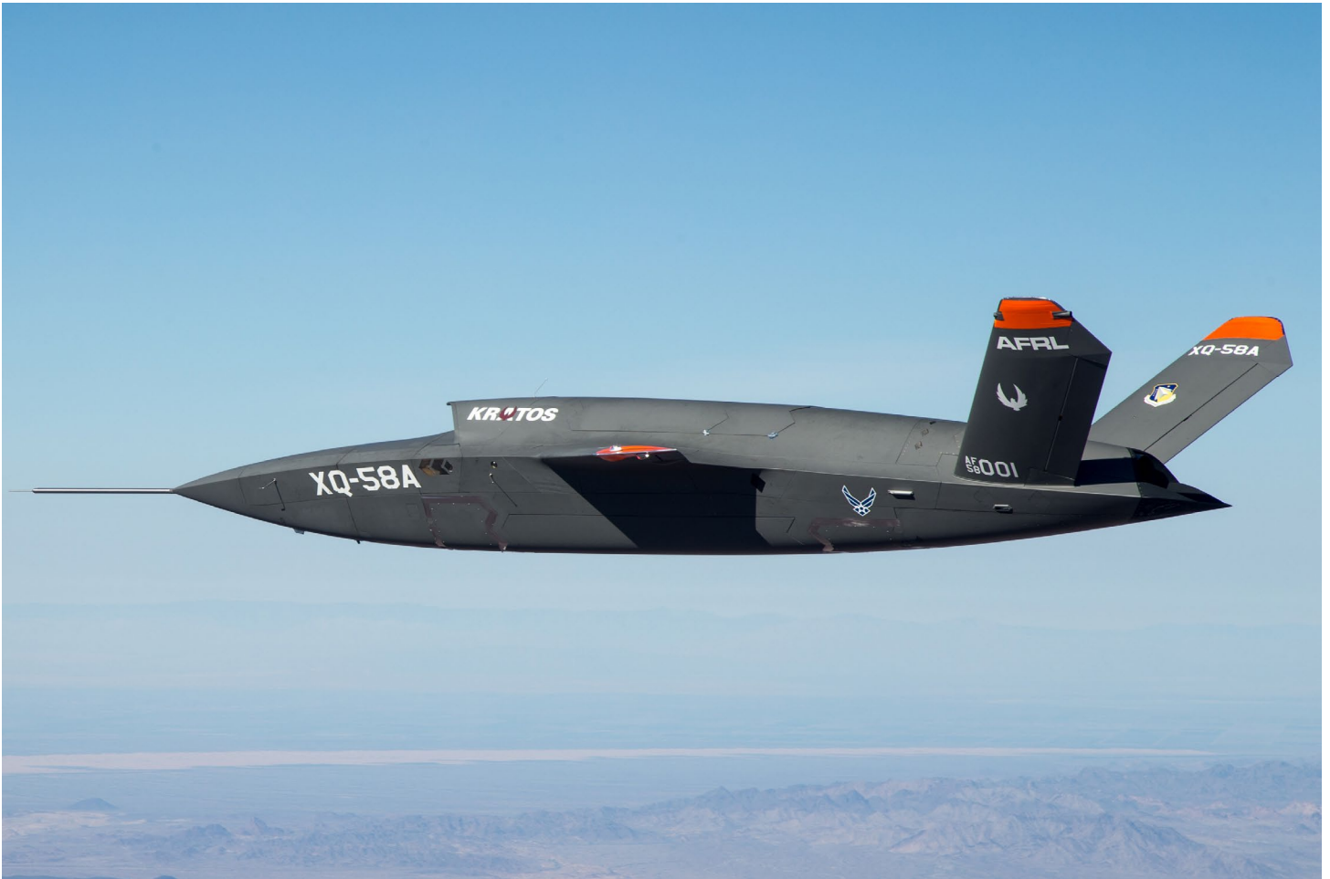
The XQ-58A Valkyrie demonstrator, a long-range, high subsonic unmanned air vehicle completed its inaugural flight March 5, 2019 at Yuma Proving Grounds, Arizona. The XQ-58A is the version of the Kratos QX222 that the US Air Force Research Lab is testing. Credit: Air Force photo by Senior Airman Joshua Hoskins
