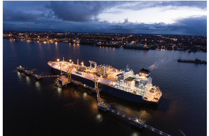
The FSRU Independence , delivered in March 2014, is an LNG carrier designed as a floating LNG storage and regasification unit used in Klaipėda, Lithuania. March 21, 2018. Wikimedia Commons/AB Klaipėdos Nafta
