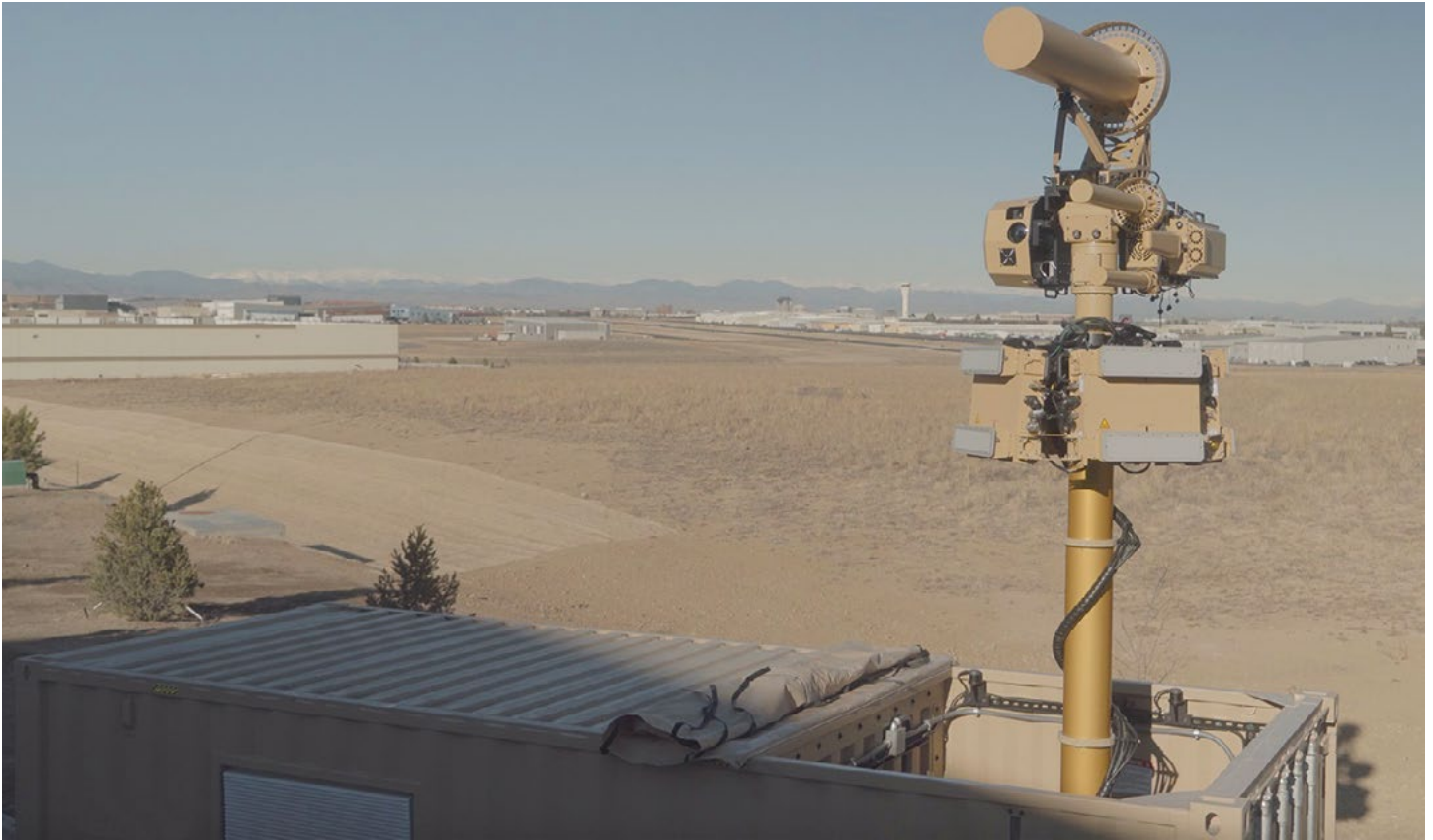
A counter-UAS system from Liteye Systems, Inc surveilles a sector near a Middle Eastern airport (May 2019). Source: Liteye Systems, Inc.
