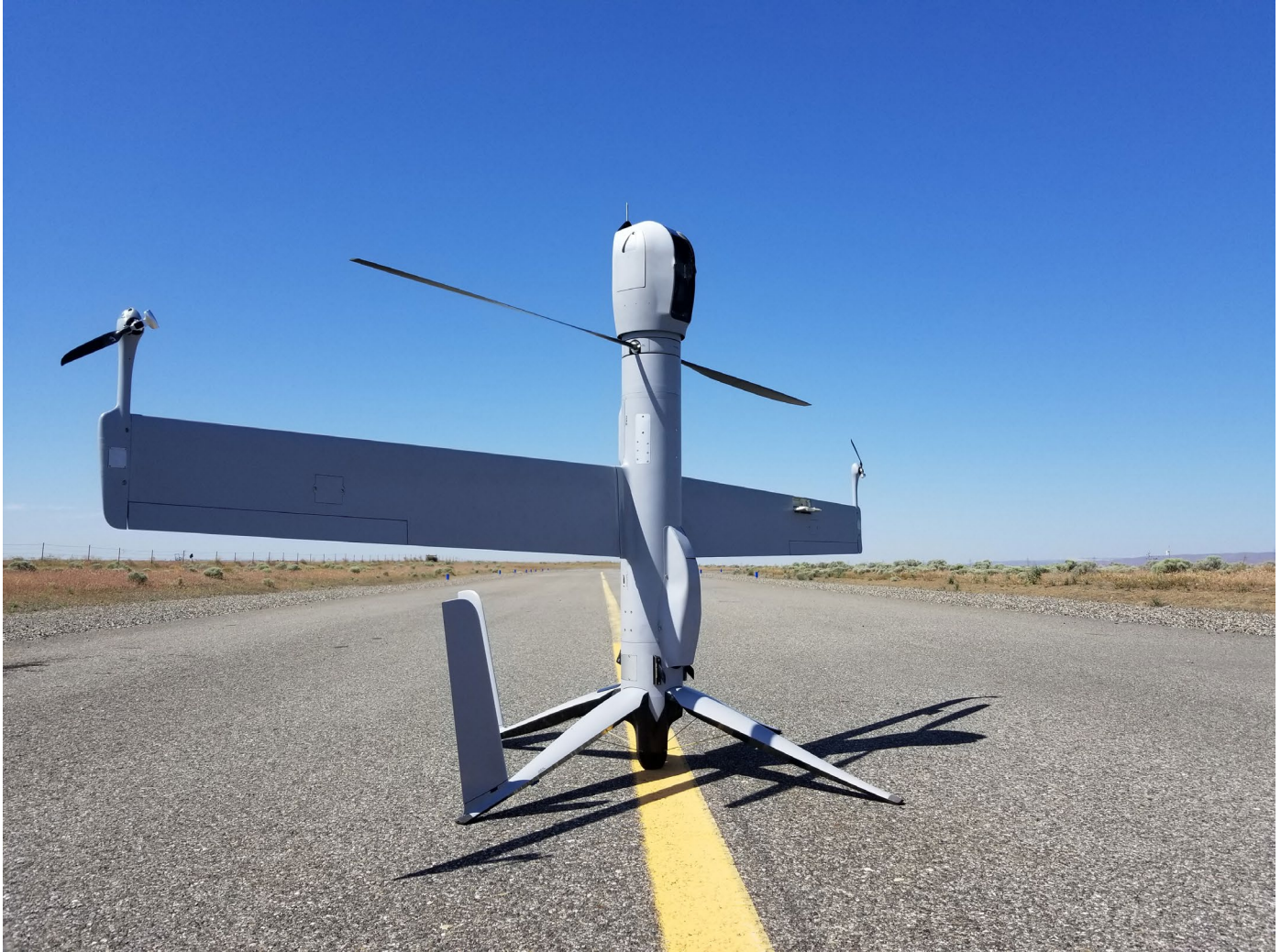
Commercial aerial drones like this Flexrotor drone are often designed to be VTOL-capable, autonomous, and long-endurance. If combined with a warhead, they are almost ideal weapons. Source: Wikimedia Commons https://commons.wikimedia.org/wiki/File:Flexrotor.jpg
