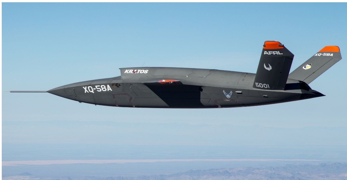
The US military is experimenting with autonomous drones like this XQ-58A Valkyrie. The major advantage of these drones is vastly reduced lifetime costs, both in operation and maintenance (O&M) costs and personnel costs. Source: Air Force photo by Senior Airman Joshua Hoskins, Wright-Patterson AFB https://www.wpafb.af.mil/News/Article-Display/Article/1777743/xq-58a-valkyrie-demonstrator-completes-inaugural-flight/
