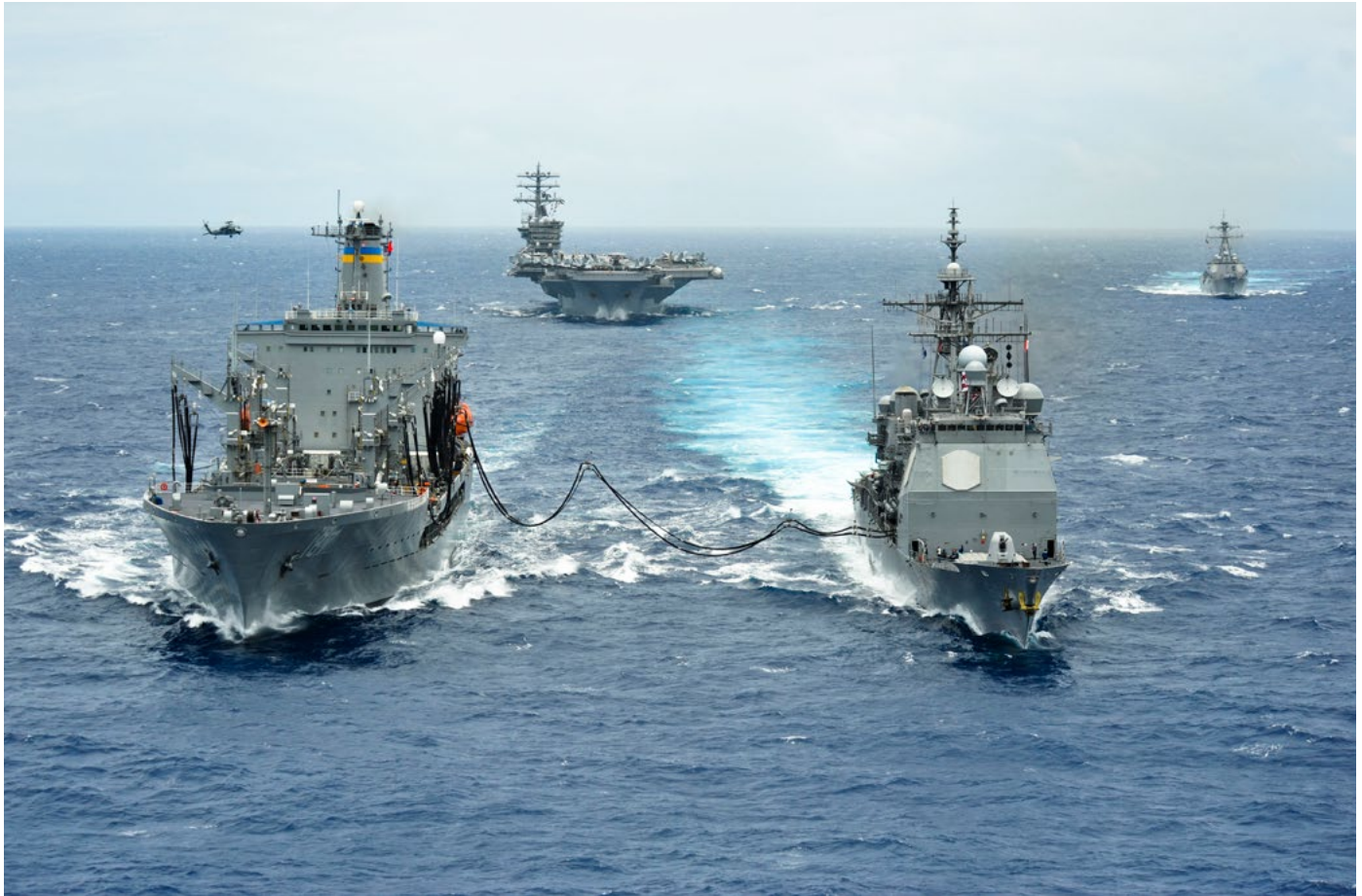
PEARL HARBOR (JULY 18, 2012) The Military Sealift Command fleet replenishment oiler USNS Henry J. Kaiser (T-AO 187), left, delivers a 50-50 blend of advanced biofuels and traditional petroleum-based fuel to the guided-missile cruiser USS Princeton (CG 59) during the Great Green Fleet demonstration portion of Rim of the Pacific (RIMPAC) 2012 exercise. In the background are the aircraft carrier USS Nimitz (CVN 68) and the guided-missile destroyer USS Chung-Hoon (DDG 93). Twenty-two nations, more than forty ships and submarines, more than 200 aircraft and 25,000 personnel are participating in the biennial RIMPAC exercise from June 29 to Aug. 3, in and around the Hawaiian Islands. The world's largest international maritime exercise, RIMPAC provides a unique training opportunity that helps participants foster and sustain the cooperative relationships that are critical to ensuring the safety of sea lanes and security on the world's oceans. RIMPAC 2012 is the 23rd exercise in the series that began in 1971. Source: Mass Communication Specialist Seaman Apprentice Ryan J. Mayes/US Navy
