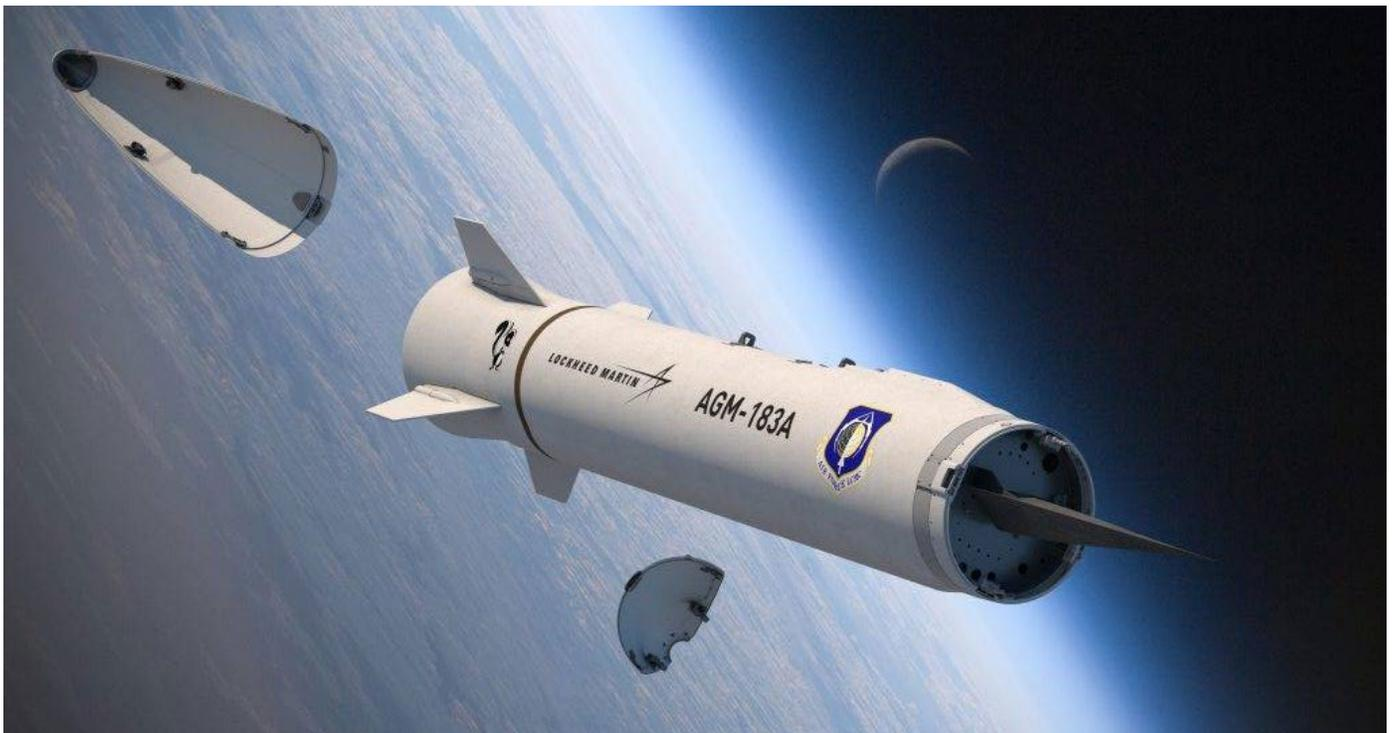
A boost-glide hypersonic weapon relies on a rocket to launch it into a low-Earth orbit, where the hypersonic projectile then detaches and glides on top of the atmosphere to its target. This design of the Air-Launched Rapid Response Weapon (ARRW) shows the rocket and projectile in low-Earth orbit prior to detachment. *Source: Lockheed Martin Corporation*
