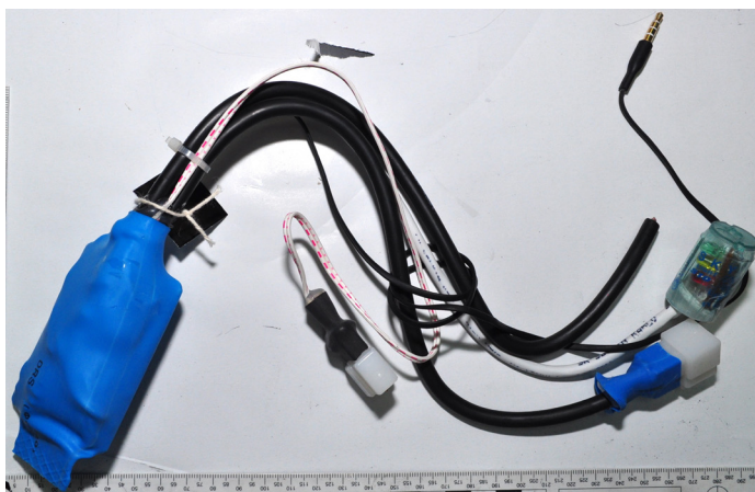
Figures 103 and 104: DTMF receiver board sealed in a blue heat-shrink wrap from the Bus Case featuring a brown-colored PCB, documented in Bahrain. 112
