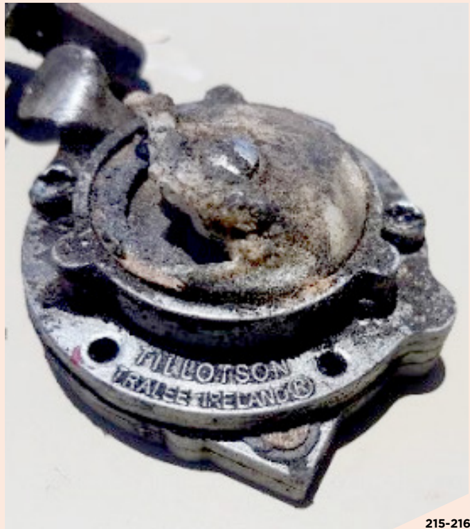
Figures 215 and 216: Tillotson-branded carburetor from a Samad-variant UAV recovered in Yemen (left) and from debris after the Aramco attack (right). 183
