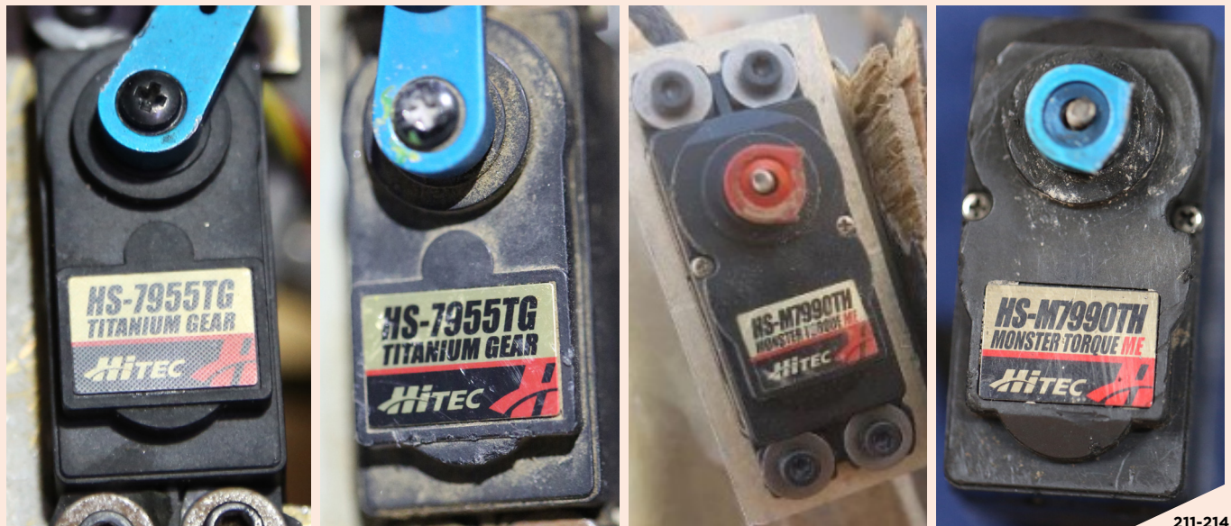
Figures 211-214: Hitec-branded servomotors documented in Qasef-1 and Samad-variant UAVs recovered from the Houthis (left and center left), recovered from debris after the Aramco attack (center right), and from a Shahed 191 UAV intercepted over Israel. 182
