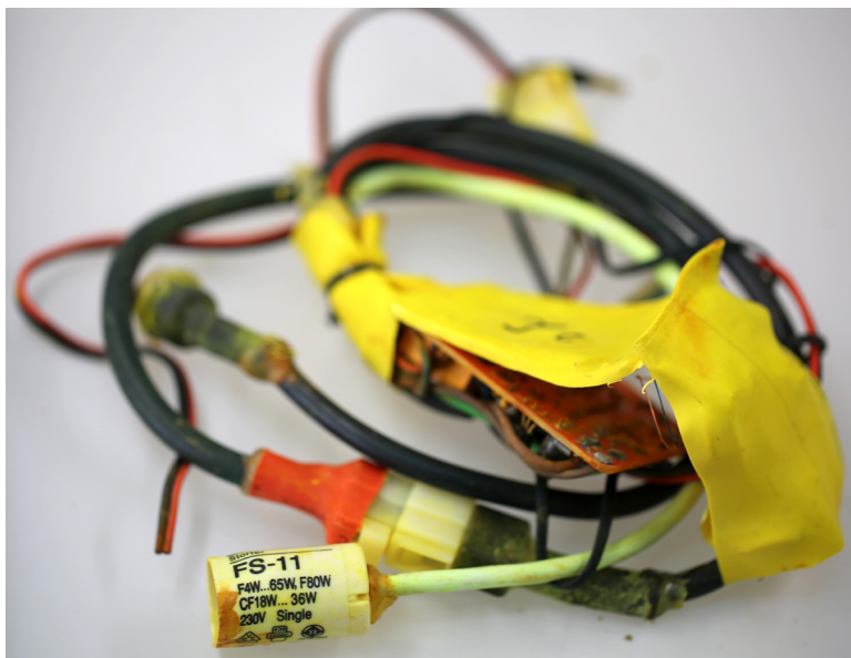
Figures 107 and 108: DTMF receiver boards featuring a brown PCB and sealed in a yellow heat-shrink wrap (left) and black heat-shrink wrap (right), documented in Bahrain. 114
