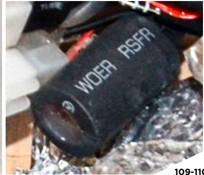
Figures 109 and 110: WOER-branded heat-shrink material on an indicator lamp connected to a DTMF receiver board (right) and DTMF receiver boards taped together with PIR sensors (left), documented in Bahrain. 115
