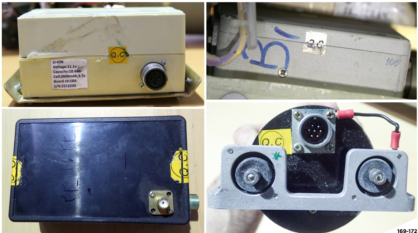
Figures 169-172: QC stickers on internal components from a Qasef-1 UAV (top, left and right), including a Bahar-branded junction box (bottom left) and V10 vertical gyroscope (bottom right), recovered from the Houthis in Yemen and documented in the UAE. 159
