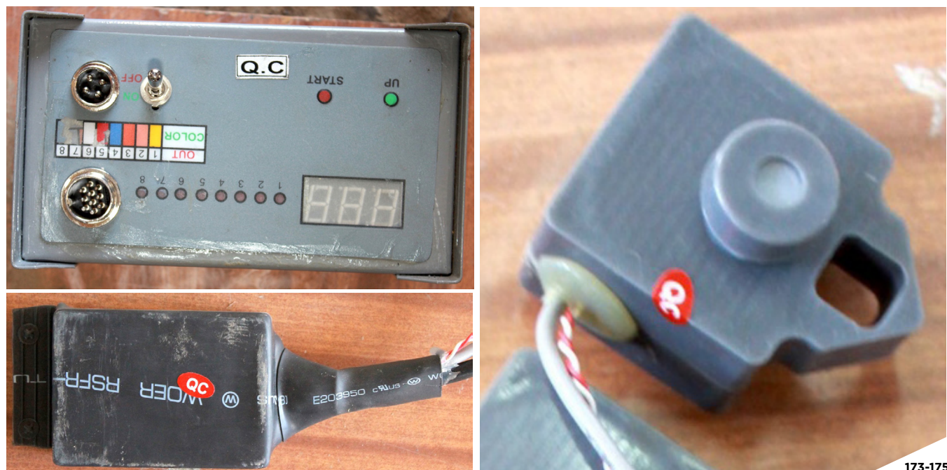
Figures 173-175: QC stickers on a control unit (top left), PIR sensor (right), and an RCIED receiver (bottom left) recovered from the Jihan 1 interdiction and documented in Yemen. 160
