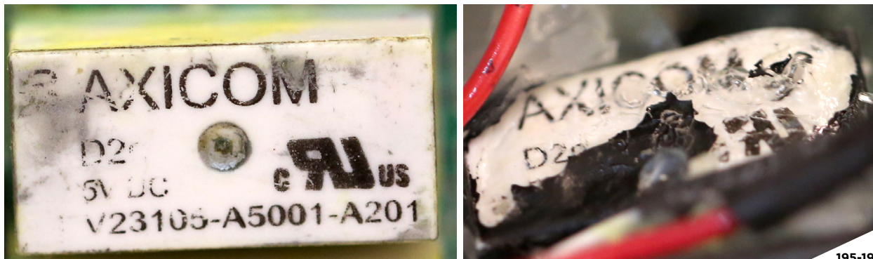
Figures 195 and 196: AXICOM-branded V23105-A50001 power relays on an RCIED receiver board contained inside a Bahar-branded junction box (left) and on an MA-RCIED receiver board (right), documented in Bahrain. 170
