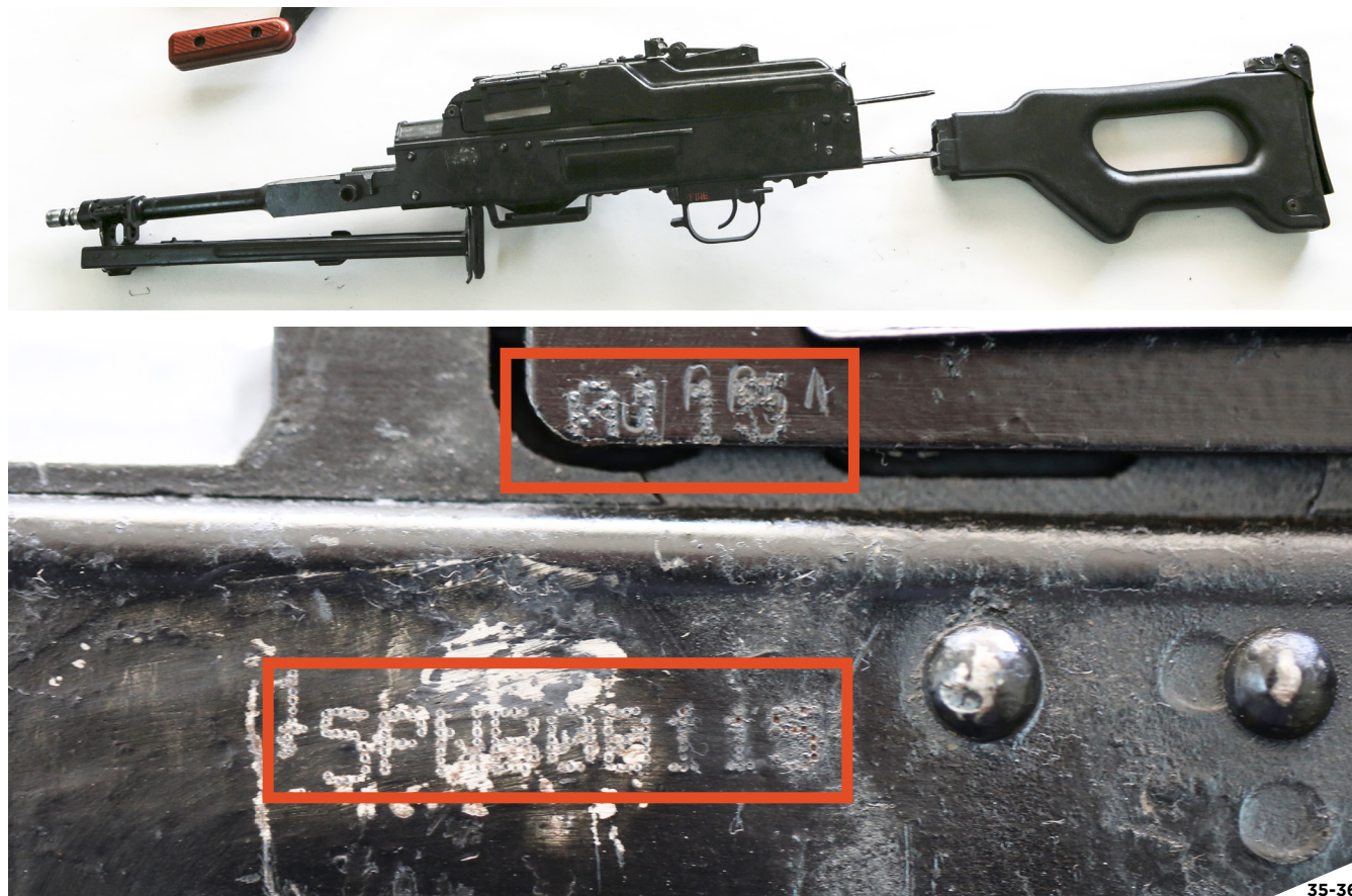
Figures 35 and 36: PKM light machine gun featuring original markings overmarked with a serial number in a format consistent with Iranian-manufactured materiel (15PNB00115), documented in Bahrain. 35
