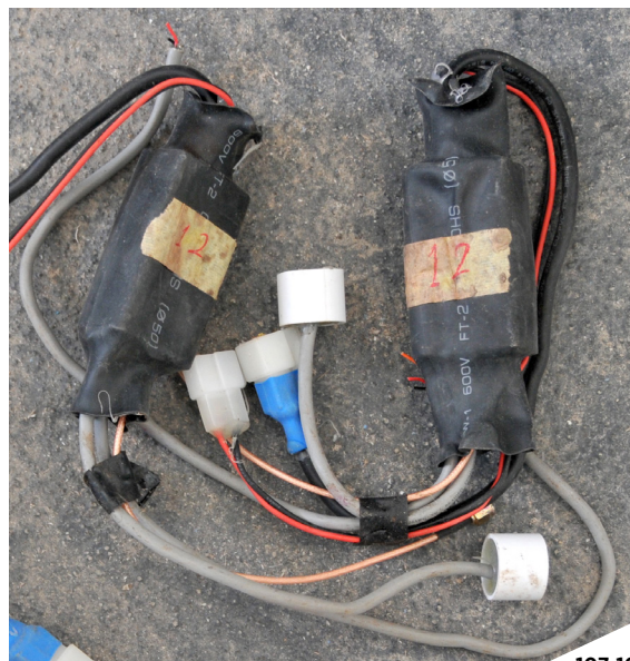
Figures 107 and 108: DTMF receiver boards featuring a brown PCB and sealed in a yellow heat-shrink wrap (left) and black heat-shrink wrap (right), documented in Bahrain. 114
