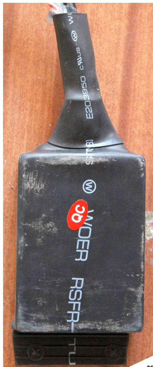
Figures 262-265: RCIED transmitter comingled with other RCIED components (top, left and right) and an RCIED programming unit (bottom), recovered from the Jihan 1 interdiction, documented in Yemen. 213
