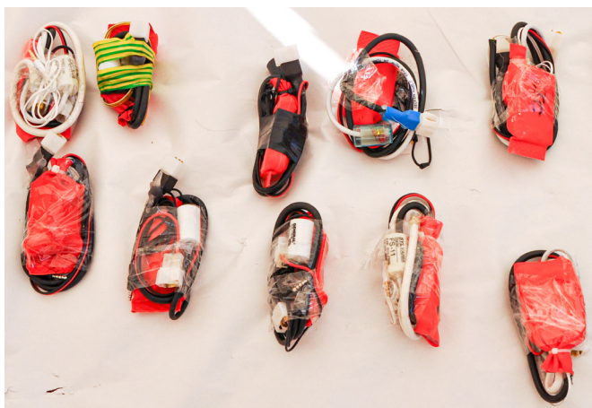
Figures 105 and 106: DTMF receiver boards sealed in an orange heat-shrink wrap and featuring brown and green-colored PCBs, documented in Bahrain. 113
