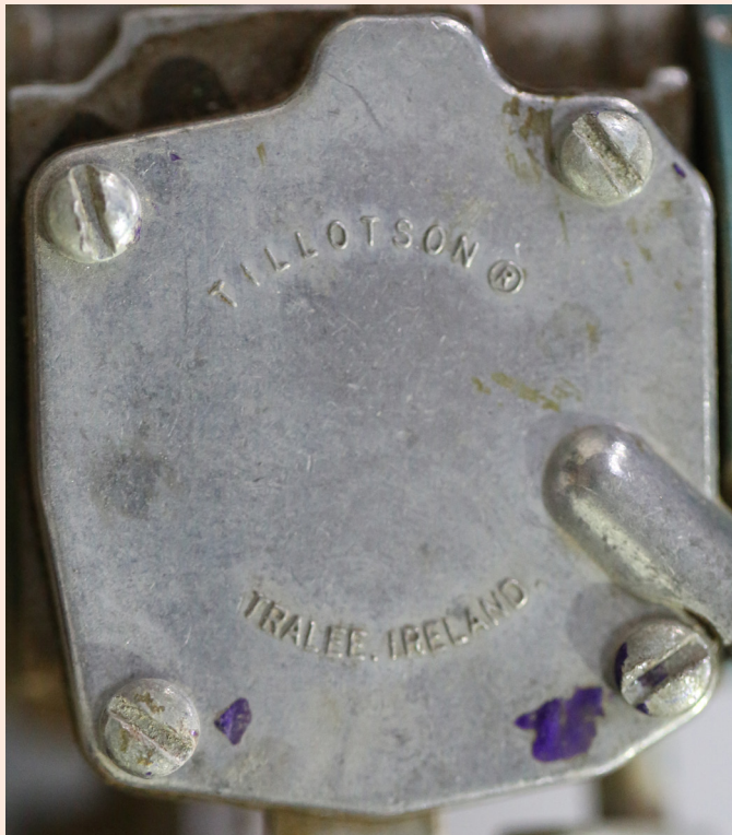
Figures 215 and 216: Tillotson-branded carburetor from a Samad-variant UAV recovered in Yemen (left) and from debris after the Aramco attack (right). 183
