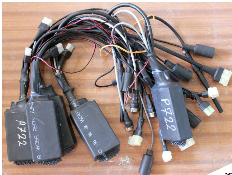
Figures 262-265: RCIED transmitter comingled with other RCIED components (top, left and right) and an RCIED programming unit (bottom), recovered from the Jihan 1 interdiction, documented in Yemen. 213
