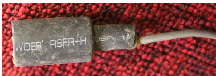
Figures 149 and 150: WOER-branded heat-shrink wire covering on RCIED receivers documented in Yemen (left) and Bahrain (right). 146
