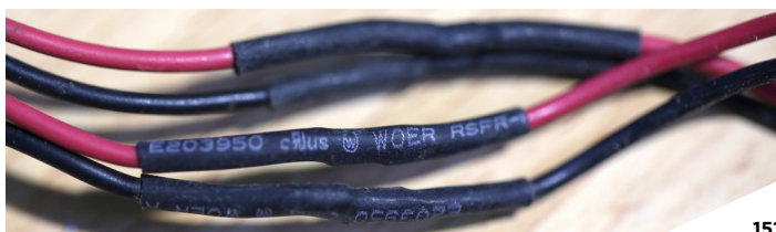
Figure 151: WOER-branded heat-shrink wire covering in an Iranian-supplied Qasf-1 UAV recovered from the Houthis in Yemen and documented in the UAE. 147
