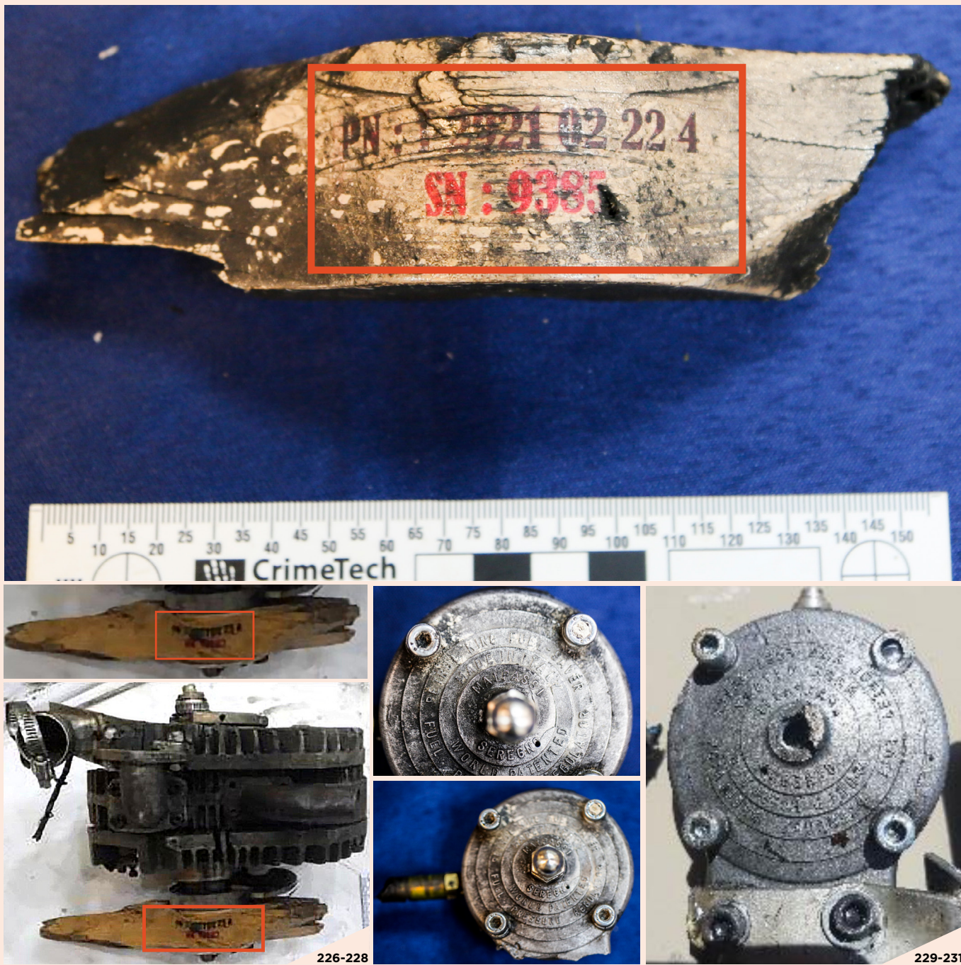
Figures 226-228: Wooden propeller recovered from a 'Shahed 191 UAV' intercepted over Israeli airspace (top) and imprinted with a serial-number pattern (in black and red ink) that is visually similar to the serial-number patterning on a wooden propeller recovered after the Aramco attack (middle and bottom). 190
