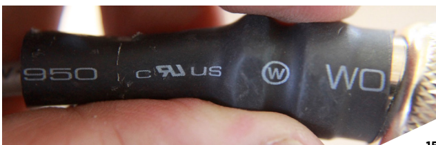
Figure 151: WOER-branded heat-shrink wire covering in an Iranian-supplied Qasf-1 UAV recovered from the Houthis in Yemen and documented in the UAE. 147
