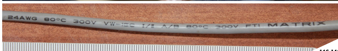
Figures 146-148: Matrix-branded wires featured on PIR sensors recovered in Bahrain (top), recovered from the Houthis in Yemen (middle), and recovered from the Jihan 1 interdiction and documented by in Yemen (bottom). 142
