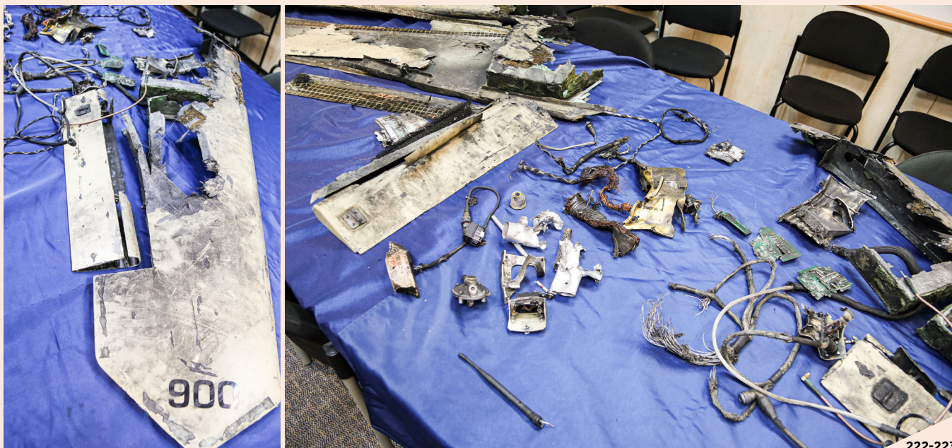
Figures 222 and 223: Debris from a ‘Shahed 191’ UAV intercepted over Israeli airspace (left and right), documented in Israel. 188
