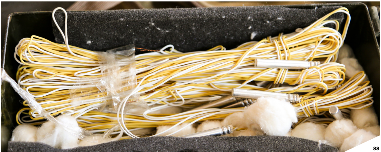
Figure 88: Commercial electric detonators with yellow and white lead wires, documented in Saudi Arabia. 96
