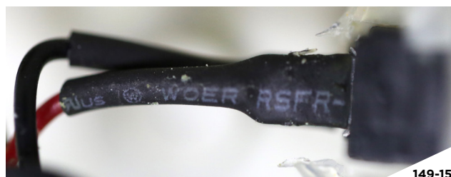
Figures 149 and 150: WOER-branded heat-shrink wire covering on RCIED receivers documented in Yemen (left) and Bahrain (right). 146
