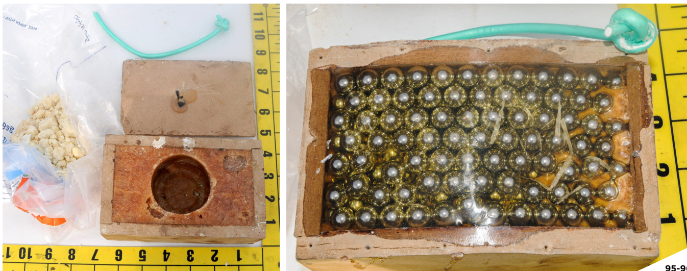
Figures 95 and 96: Improvised directional mine documented in Bahrain (left and right). 102
