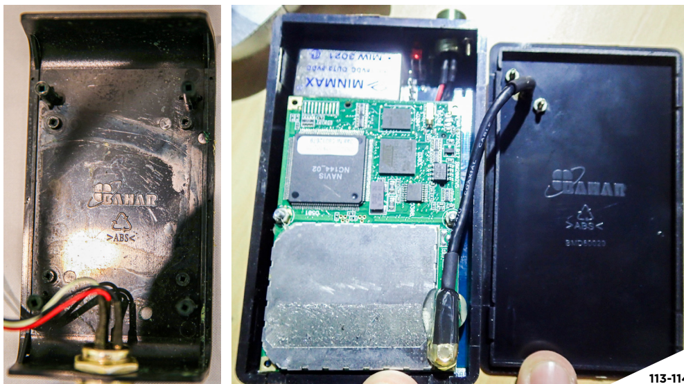
Figures 113 and 114: Bahar-branded junction boxes containing an RCIED receiver board documented in Bahrain (left), and inside an Iranian-supplied UAV recovered in Yemen, documented in the UAE (right). 120
