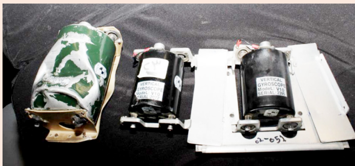
Figures 217-221: Vertical gyroscopes recovered from a Qasef-1 UAV in Yemen (top left), an Ababil-3 UAV in Iraq (top center), debris after the Aramco attack (top right), displayed at the Iranian Military Display in Washington, DC (bottom left), and documented in a SAM recovered from the Forest Sherman interdiction (bottom right). 184
