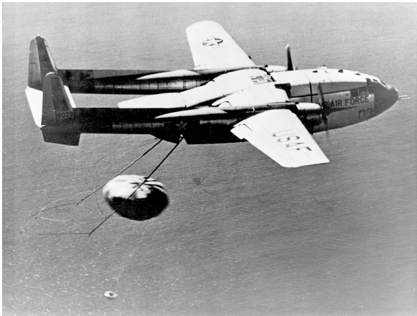
US Air Force C-119J recovers a CORONA capsule returned from space. Source: US Air Force
