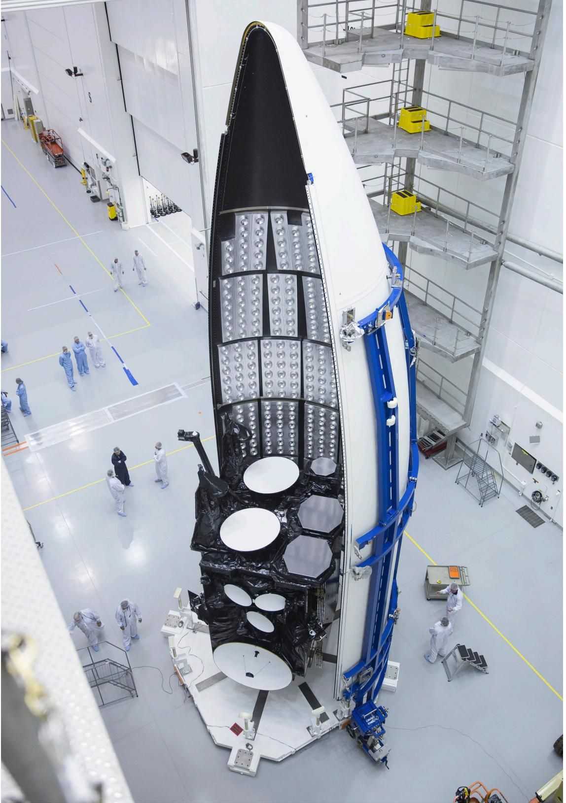
As adversarial nations obtain new capabilities to disrupt US and allied satellites, the United States must ensure resilient space systems. In this picture, workers prepare the US Air Force Advanced Extremely High Frequency satellite, which provides survivable, near worldwide, secure, protected, and jam-resistant communications for high-priority national military operations.
