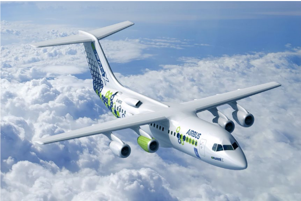
Airbus' E-Fan X aircraft is an example of the aerospace industry's efforts to harness electric propulsion as means of air travel Source: Airbus
