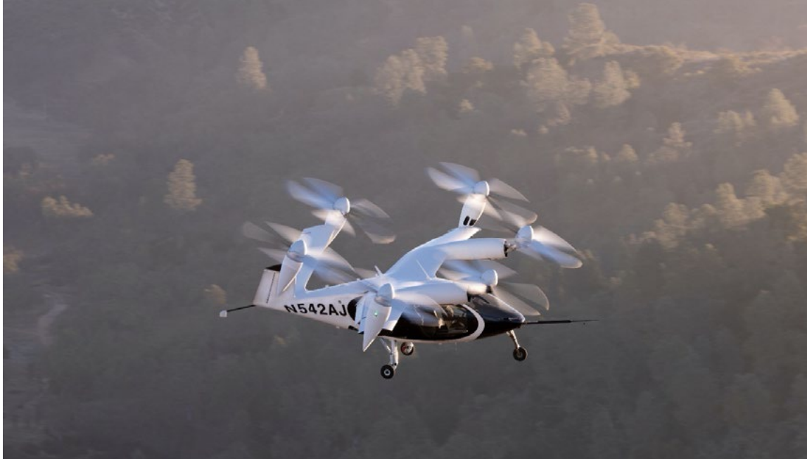
A Joby Aviation electric vertical take off and landing (eVTOL) personal aircraft is seen on a test flight Source: Joby Aviation
