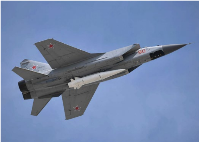
Russia's Kh-47M2 Kinzhal is a dual-capable hypersonic weapon shown here on a MiG-31 interceptor. It is featured here in the 2018 Moscow Victory Day Parade. Source: by courtesy Russian Presidential Press and Information Office.
