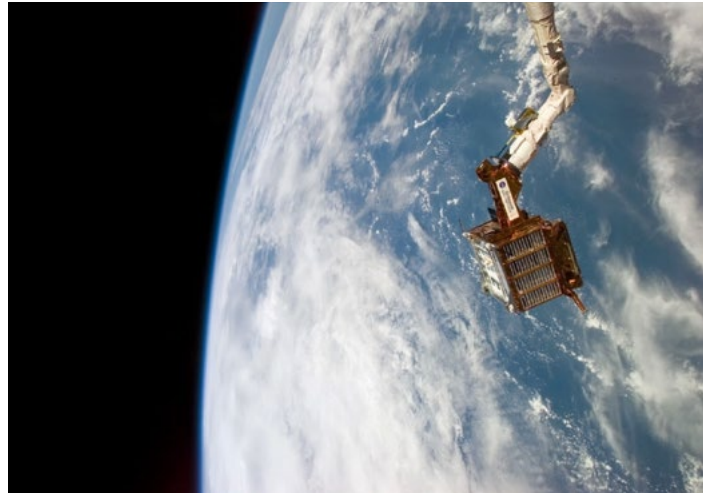
View of the SPARTAN 201 satellite on the Remote Manipulator System (RMS) arm end effector, during retrieval of the satellite. Source: NASA, December 15, 2010.
