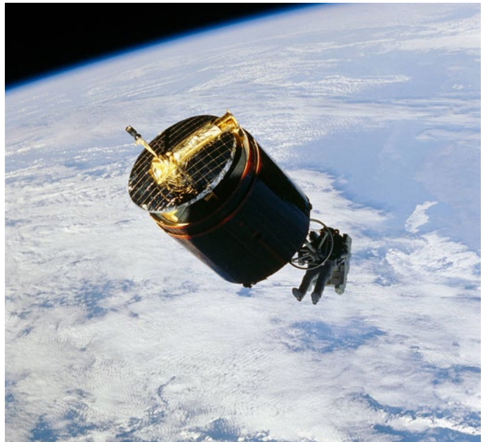
Astronaut Dale A. Gardner, getting his turn in the Manned Maneuvering Unit, prepares to dock with the spinning WESTAR VI satellite during the STS-51A mission. Source: NASA, August 7, 2017, https://www.nasa.gov/audience/foreducators/spacesuits/historygallery/shuttle-nov84a.html
