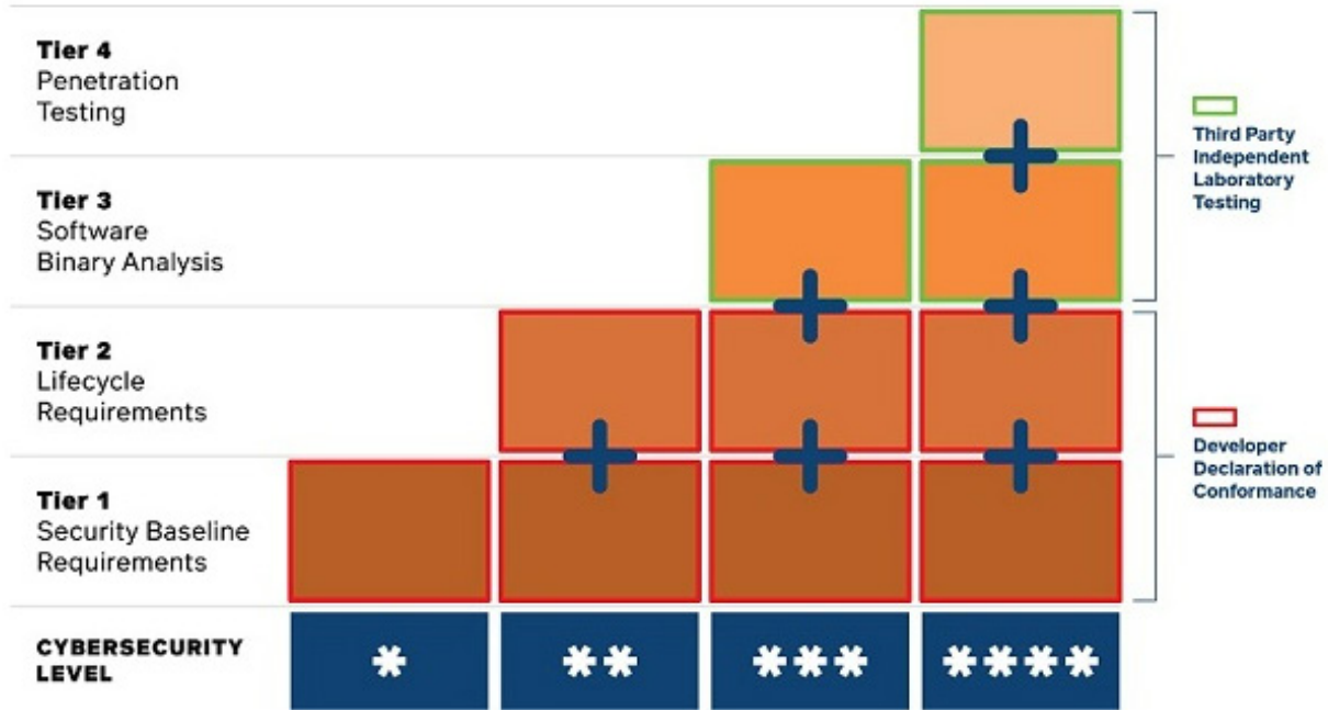
Figure 2: Singapore’s CLS Four Security Provisions Tiers
