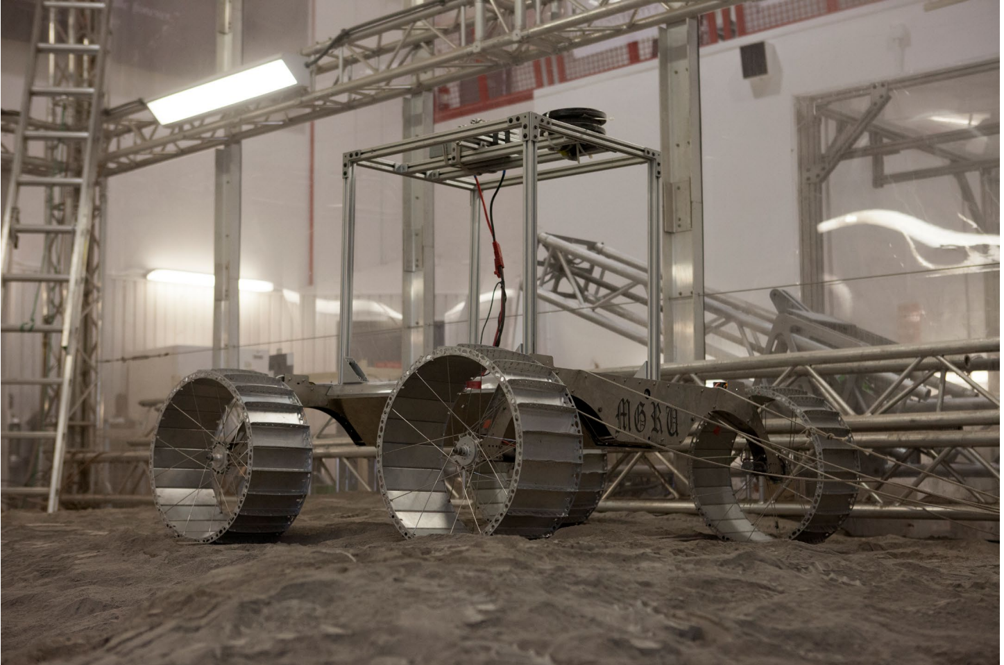
A lightweight simulator version of NASA's Resource Prospector undergoes a mobility test in a regolith bin at the agency's Kennedy Space center in Florida. The Resource Prospector mission aims to be the first mining expedition on another world. Source: NASA/Kim Shiflett, https://commons.wikimedia.org/wiki/File:KSC-20170628-PH_KLS01_0073_(35596106876).jpg .
