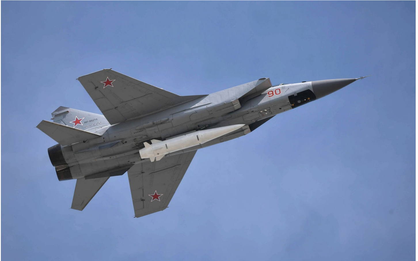
Russian MiG-31 'Foxhound' supersonic interceptor jet carrying an anti-satellite weapon during the 2018 Victory Day Parade. Source: kremlin.ru, https://commons.wikimedia.org/wiki/File:2018_Moscow_Victory_Day_Parade_66.jpg .
