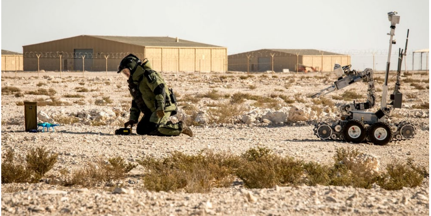
An officer places an XRS-150 X-ray generator in front of a simulated downed unmanned aerial system. Credit: US Air National Guard, Brigette Waltermire https://www.dvidshub.net/image/6485647/379th-esfs-and-eod-team-up-counter-uas-training .
