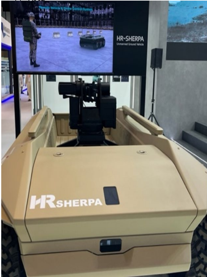
A Hyundai Rotem HR-Sherpa uncrewed ground vehicle on display at the International Defence Exhibition & Conference in Abu Dhabi in February 2023. The image behind and above the vehicle demonstrates one operational concept in which a human operator controls and works in tandem with the Sherpa. Training and trust are required to ensure that these concepts are designed and executed in ways that effectively exploit the advantages of HMT. Image: Tate Nurkin
