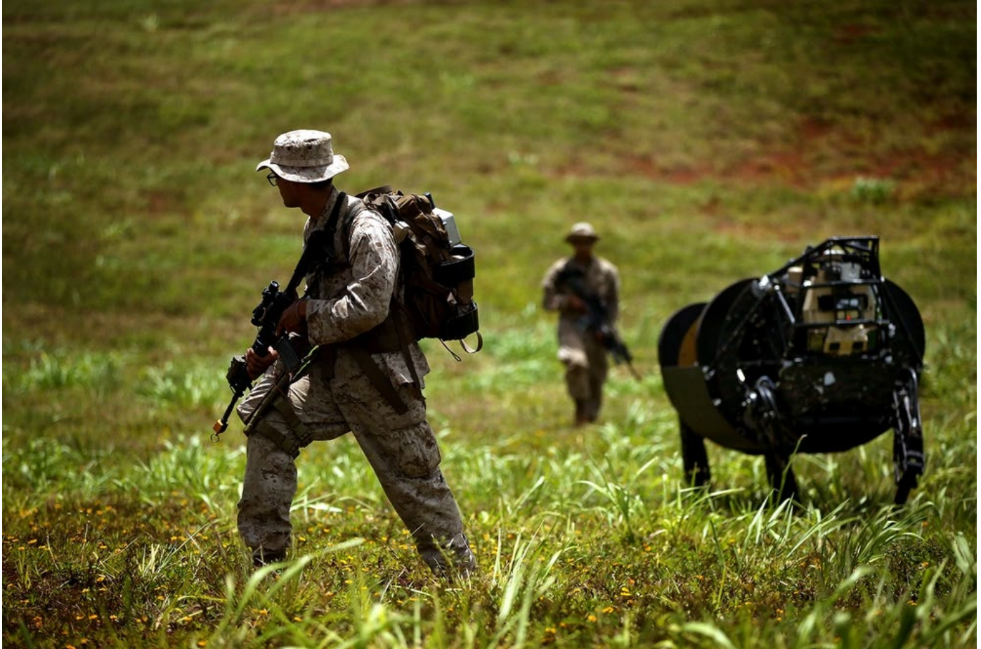
The Legged Squad Support System is experimental technology being tested by the Marine Corps Warfighting Lab. It is programmed to follow an operator through terrain, carrying heavy loads like water and food. Credit: US Marine Corps, Matthew Callahan: https://www.dvidshub.net/image/1445811/meeting-ls3-marines-experiment-with-military-robotics .
