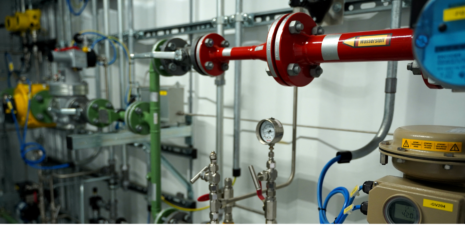
A gas blending station tests a mixture of hydrogen and natural gas. REUTERS/Timm Reichert.
