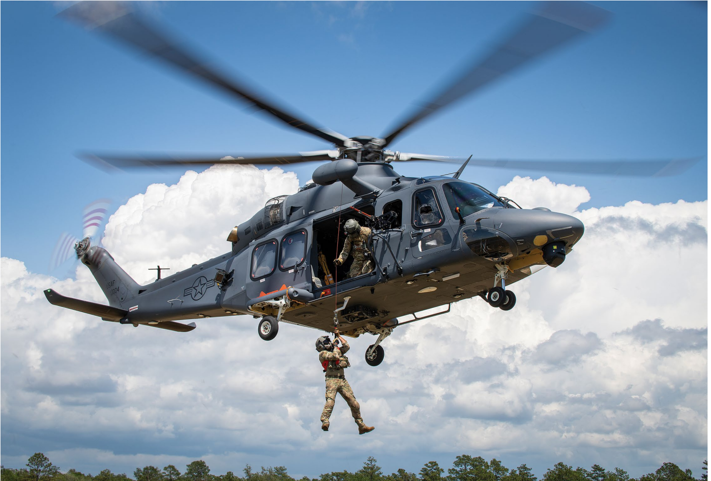
A MH-139A Grey Wolf's successful live hoist test. Photo by Samuel King Jr. 96th Test Wing Public Affairs.
