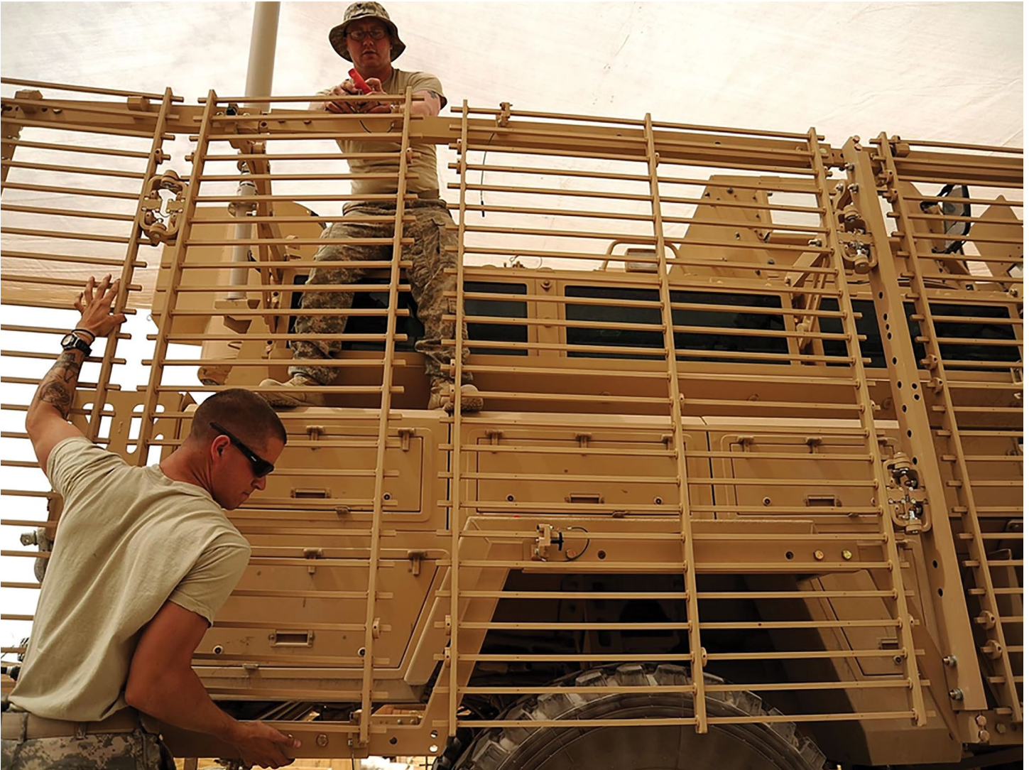
Soldiers connect L-Rod Bar Armor to an RG-31 Mine Resistant Ambush Protected vehicle at Kandahar Airfield, Afghanistan. Photo by Staff Sgt. Stephen Schester, 16th Mobile Public Affairs Detachment.
