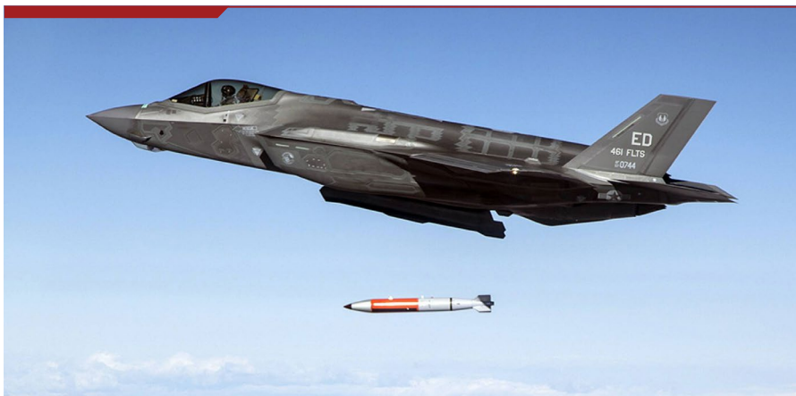
A US F-35 fighter jet dropping an inert B61-12 gravity bomb in a test of the device, December 2021.
