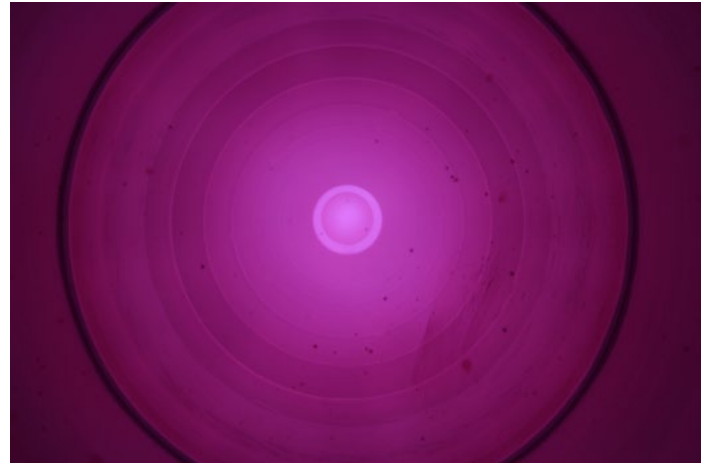
An end-on view of Helion Energy's sixth-generation fusion prototype shows a fuchsia glow, which comes from the hydrogen Balmer series (emission of visible light due to excitation and recombination). Source: Helion Energy
