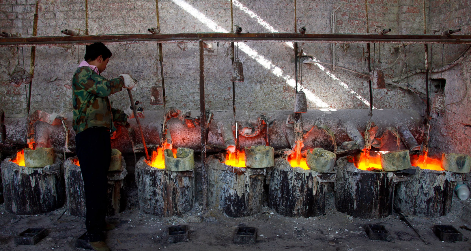
A worker at the Jinyuan Company's smelting workshop in China's Inner Mongolia Autonomous Region stokes the pots containing the rare earth metal lanthanum. REUTERS/David Gray.
