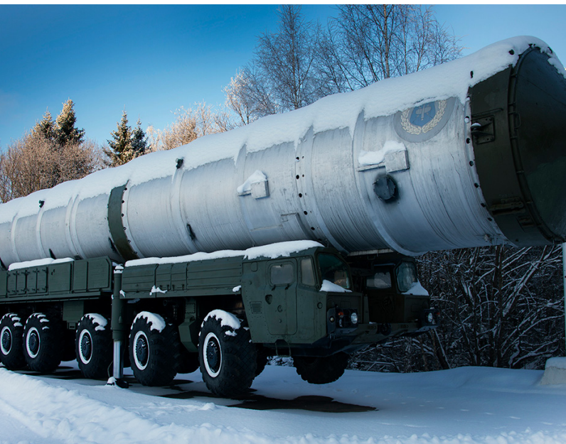
A transport and reloading vehicle on the for 51T6 long-range interceptor missiles as part of the A-135 Amur anti-missile defense complex (Yuriy Shipilov, Ministry of Defense of the Russian Federation)
