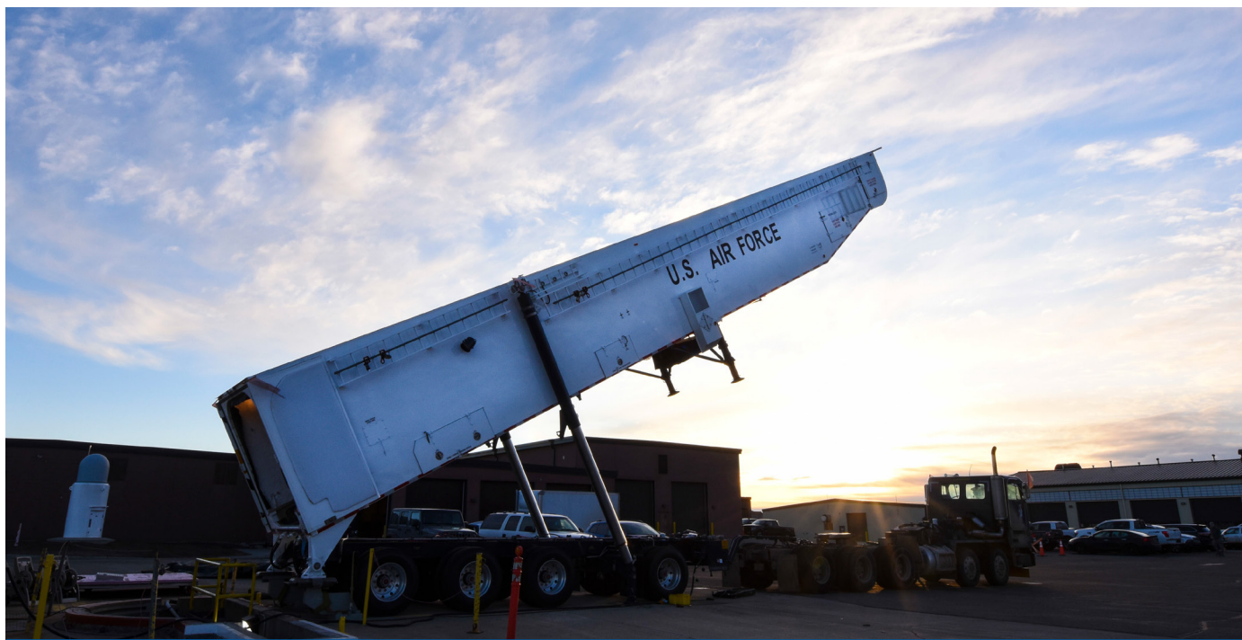
Transporter erector is raised during an annual proofload test at Minot Air Force Base, North Dakota, April 2, 2019 (US Air Force photo by Senior Airman Ashley Boster).
