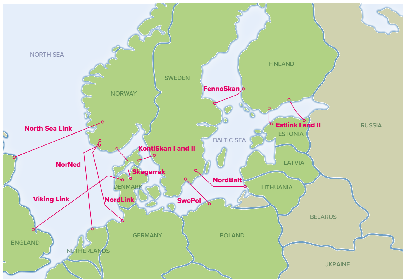
Figure 3: Undersea electricity interconnections in Northern Europe
